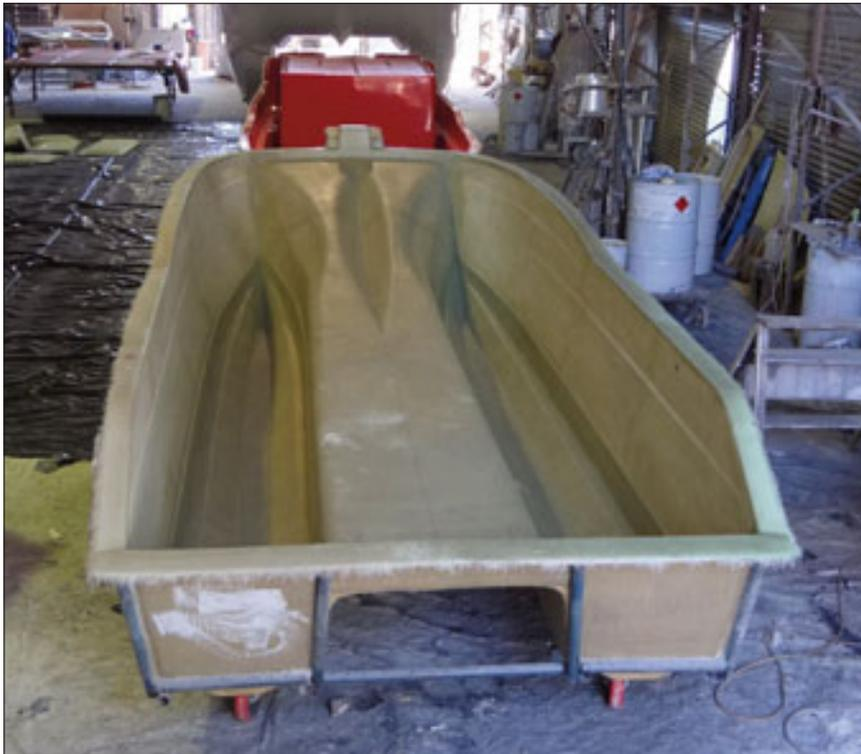
**Above:** The Voyager 625 uses conventional fibreglass technology in a beautifully built set of moulds, to achieve an unusually high standard of inherent, 'off the gun' finish. Build time is usually 6-8 weeks from order.
