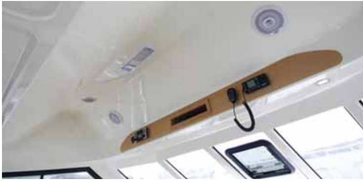
The raised roof level was a novel way of enhancing the apparent size and volume of the saloon.
