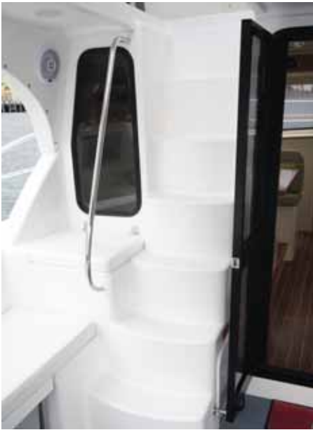
Clever design saw a set of moulded steps take up no more room than a ladder. (above left)
